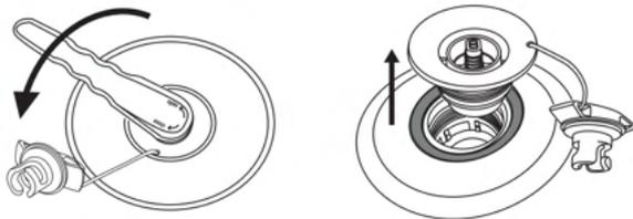
3. Check the rubber ring to make sure that it is in the correct position, tight around the valve without any debris.
