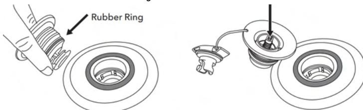
4. Make sure the pin spring is functional and does not have any cracks. Also make sure there are no strings from the stitching material in the way.
